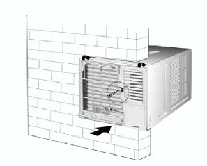
• Attach the air filter to the front grille.
